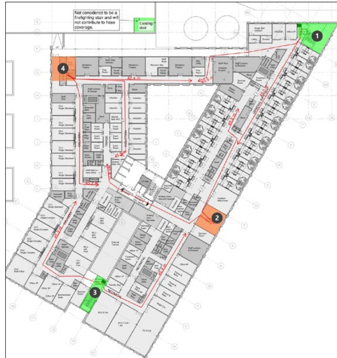
Figure 8: Hose coverage - potential relocated stair positions
